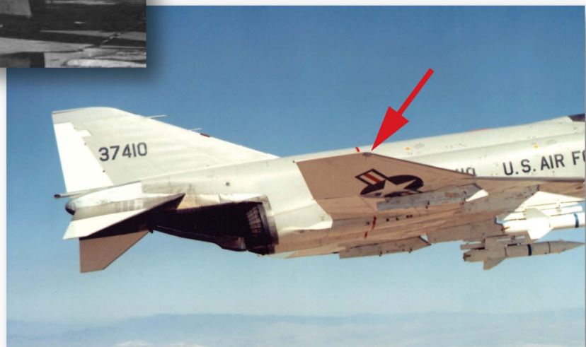
Right: F-4C-15-MC 63-7410 showing the flush style lights.
