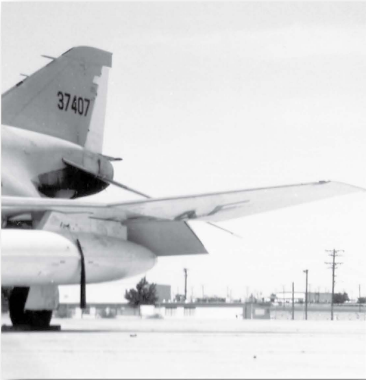
Above: F-4C-15-MC 63-7407 displays the flush style light shortly after roll out in July 1963.
