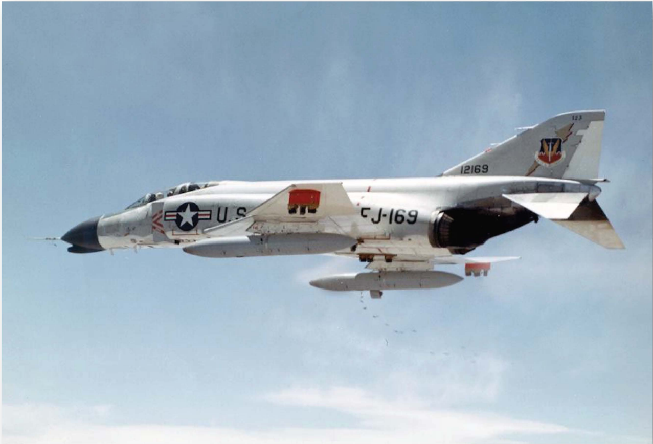
As noted above, photos of the two F-110A prototypes after they officially became F-4Bs and received their USAF serial numbers are very rare. But we found this superb shot of the second F-110A, now F-4B 62-12169, line number 123. Most likely taken near Holloman AFB during 1963 while she was deeply involved in weapons testing. She's loaded with a pair of early SUU-16/A 20mm gun pods (note the fully faired, tapered noses on the pods), and has a very draggy looking camera setup dangling from under both wing tips and on the fuselage. Note the air data boom on the nose. She appears to retain the dark yellow lightning bolt. This would make a fantastic looking model!
