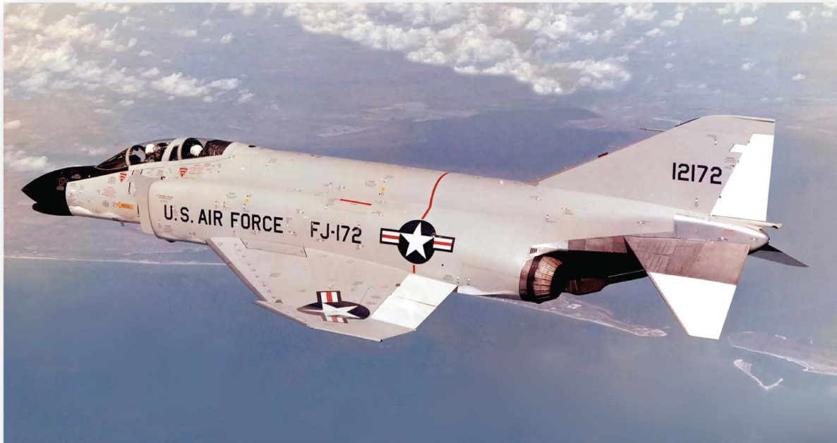
F-4B-14-MC 62-12172 (Navy BuNo 150480), the first of 27 operational F-4Bs assigned to the 4453rd Combat Crew Training Squadron at MacDill AFB, Florida. Her markings are 100% standard, albeit lacking the TAC lightning bolt badge. Note the yellow hoist point markings now applied in the early USAF style, the black anti-glare panel, and her overall pristine appearance. She served a long career in the USMC, and was eventually converted to an F-4N, and retired in 1983. See photo on page 21.
