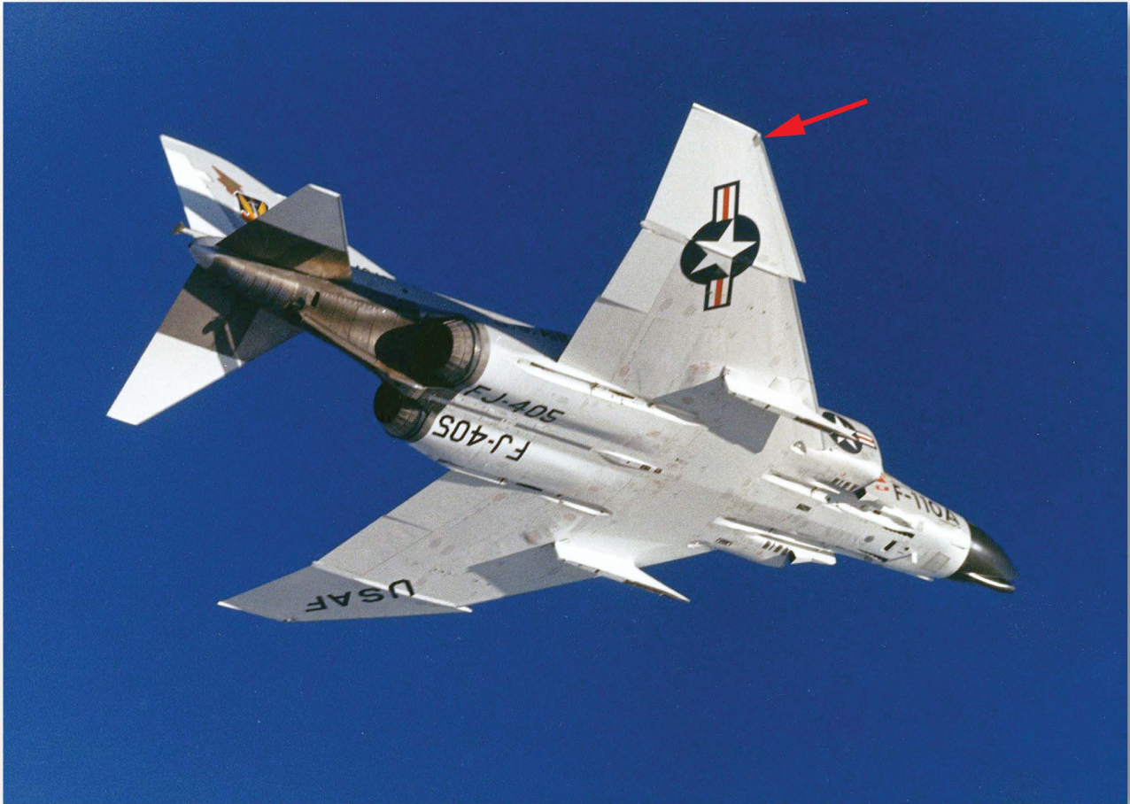
This gorgeous shot of F-110A 149405 illustrates her USAF markings well. Note the natural metal strips along the fuselage keel between the buzz numbers. You can just make out the early style flush wing tip navigation light, indicated by the arrow. The 25" USAF wing titles on these early aircraft were located further outboard than the later standard. The dark yellow TAC lightning bolt is shown to advantage here.
