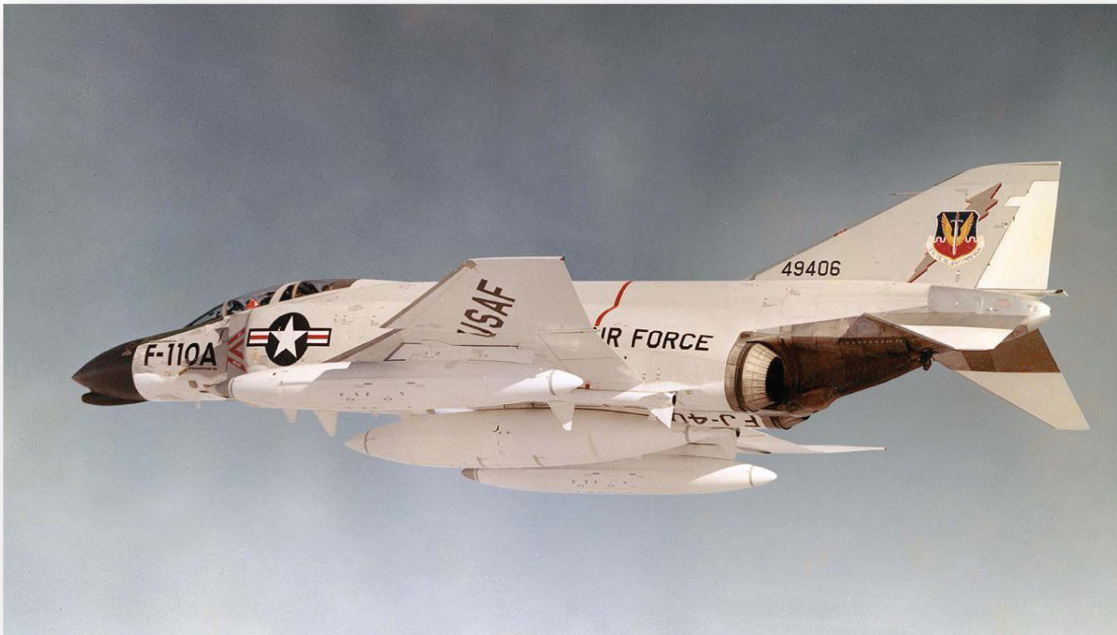
F-110A 149406. Note the position of the USAF titles on the wings, as well as the relatively shiny silver Corogard paint above the horizontal stabs and on the tail cone. The TAT probe is just visible above the first “4” of the tail number. In common with every F-4 produced, the translating ring forward of the exhaust petals is painted glossy black. The lack of sooty black exhaust staining indicates the aircraft has very little flight time on her clock, or else someone at McDonnell spent a lot of time cleaning her up!
