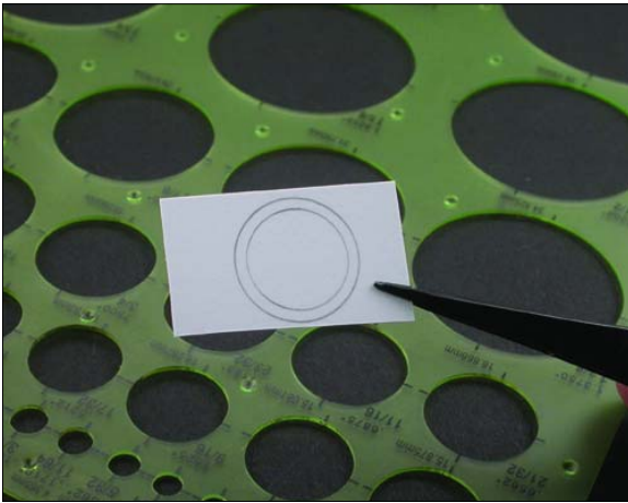
This photo shows how to make a small ring or disc. As you can see a smaller inner circle has been added to a larger outer one.
