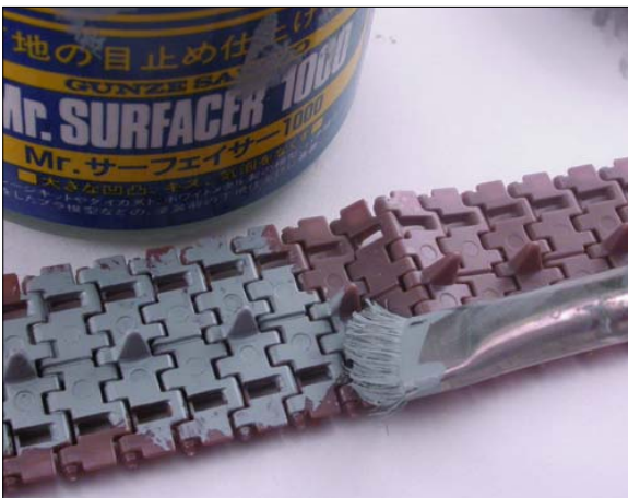
A couple of quick stippled coats of Mr Surfacer 1000 can cover the 'knock-out' marks – better than sanding every track individually!
